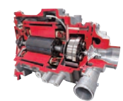
Air Compressor used in the Mirai
