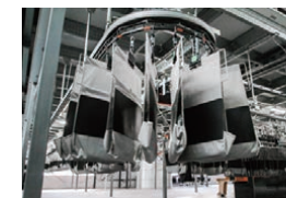
VANDERLANDE Hanging Type High-Speed Sorting System Pocket Sorter
