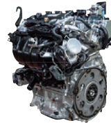
A25A-FKS Displacement: 2.5 liters used in the RAV4
